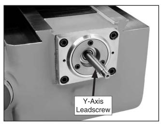
**Figure 66.** Ball handle, ring, and key removed from Y-axis leadscrew.
